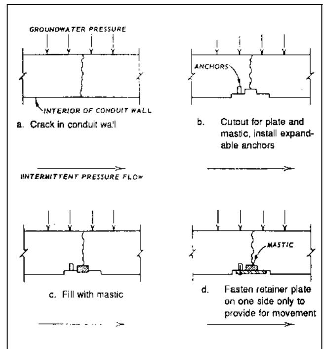
Figure 6-8. Repair of crack by use of a retainer plate to hold mastic in place against external pressure
