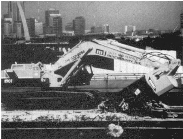
**Figure 5-2. Boom-mounted concrete crusher**
